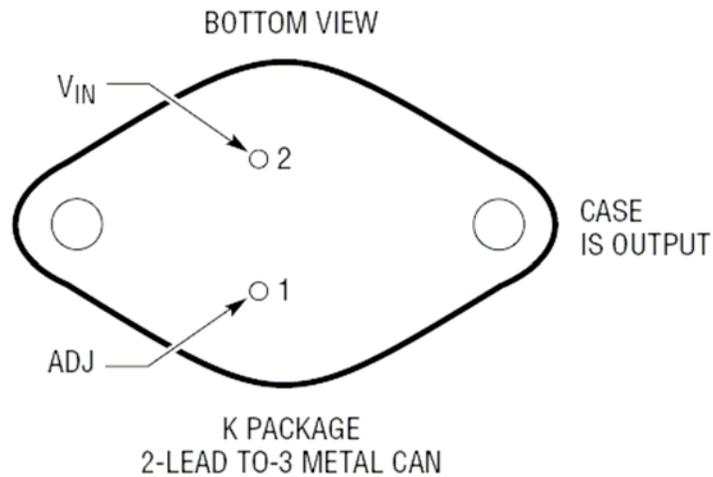
Figure B.2. K package drawing (for reference only). This figure was extracted from the LINEAR TECHNOLOGY CORPORATION RH117 Datasheet.
